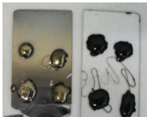
Figure 4. Bitumen sample, before (right) and after (left) preparation for being placed under microscope (the left sample: placing in vacuum chamber and covering with a thin layer of gold)
