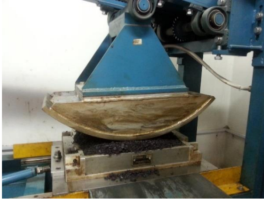
Figure 1. Asphalt mixture compaction
