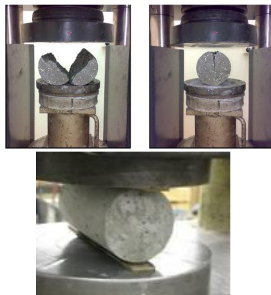
Figure 3. Cylindrical sample in the splitting test
