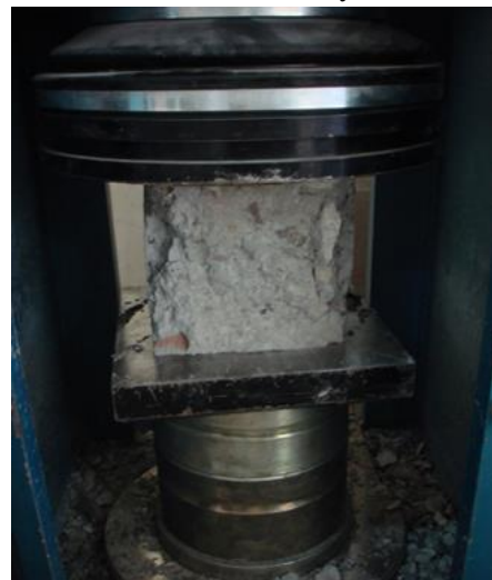
Figure 2. Cubic sample under compression test and the satisfactory state of rupture of the tested samples
