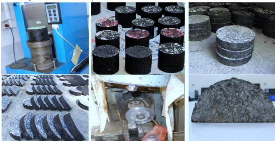
Figure 3. Steps for preparing SCB samples
