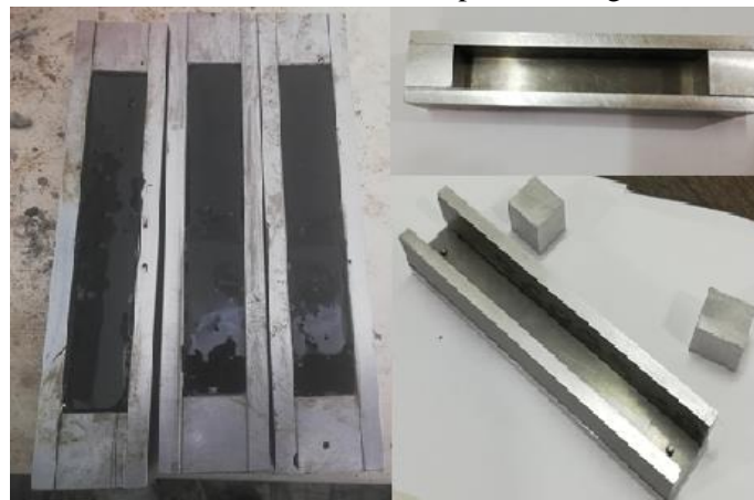
Figure 4. Molds made for preparing the binder specimens
