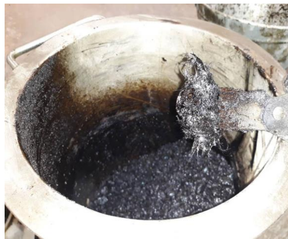
Figure 9. A picture of fiber agglomeration when excessive fiber length or content is used
