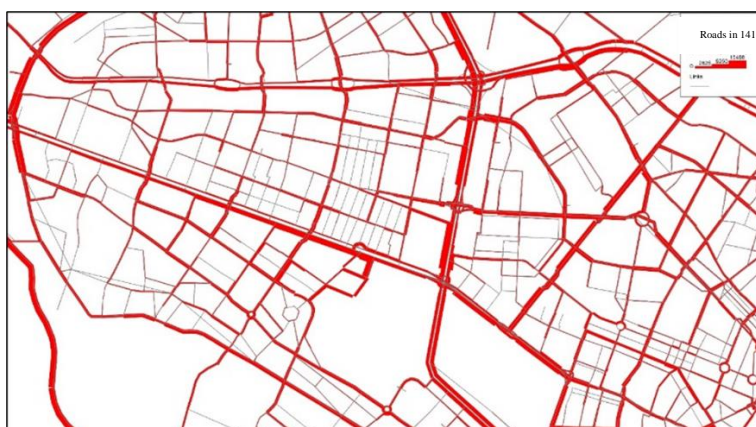
Figure 17. traffic volume passing through the roads in the base scenario (do nothing)
