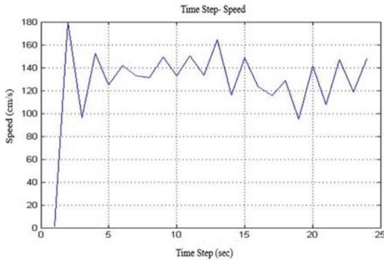
**Figure 8. Final speed of a pedestrian in presence of 21 other pedestrians with certain initial distances**
