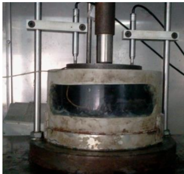
Figure 3. Saturated specimen inside the water container during the dynamic creep tests
