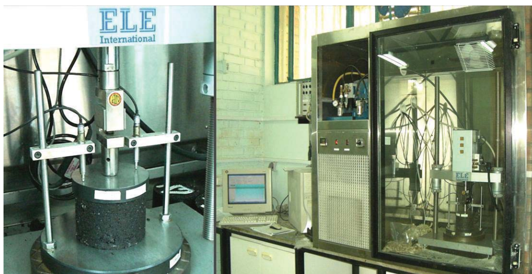
Plate. 1. UTM (right) and specimen mounted in the machine for dynamic creep test (left) (Asphalt and Bitumen Research Center, Iran University of Science and Technology)
