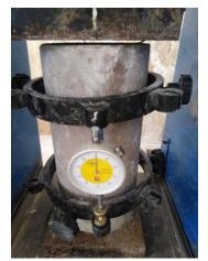
Figure 6. Concrete Specimen Undergoing Modulus of Elasticity test
