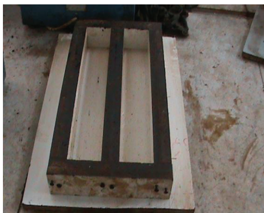
(a) Molds for making beam specimens
