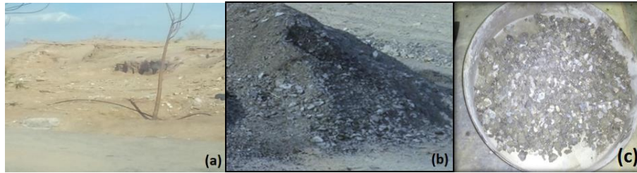
Figure 1. a) The location of preparing the subgrade sandy aggregates and b) The deposit of RAP aggregates c) Used RAP aggregates
