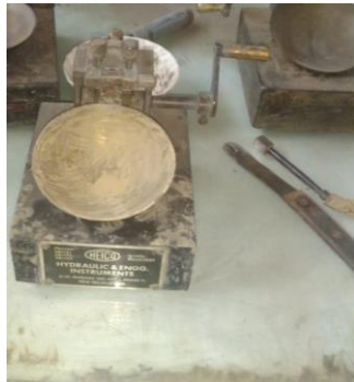
(a) Liquid Limit Test
