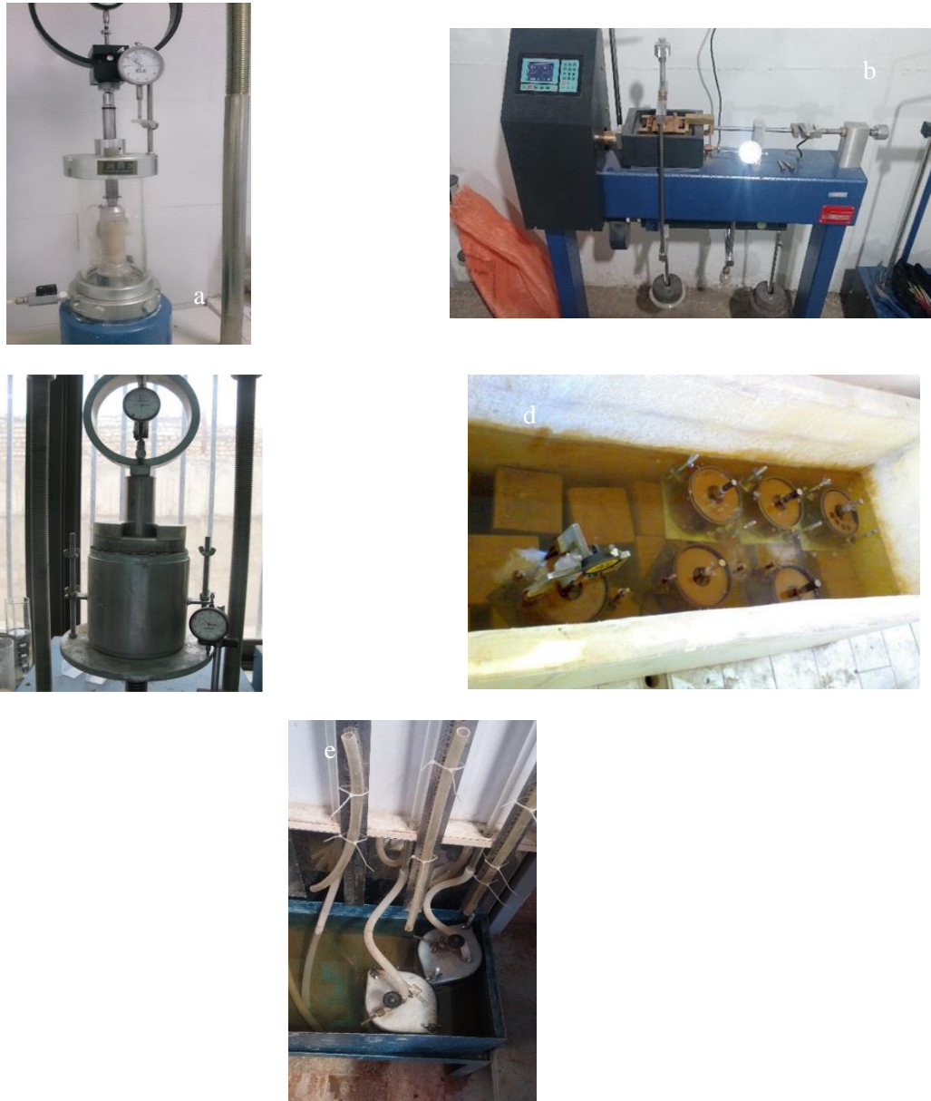
Figure 3. Test apparatus used in the present study: (a) Uniaxial compressive strength test; (b) Direct shear test; (c) CBR test in a dry condition; (d) CBR test in a saturated condition; (e) Falling head permeability test
