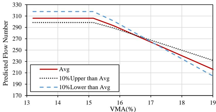
Figure 6. The effect of voids in mineral aggregate on the flow number of asphalt mixtures
