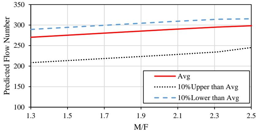
Figure 7. The effect of Marshall stability to flow ratio on the flow number of asphalt mixtures.
