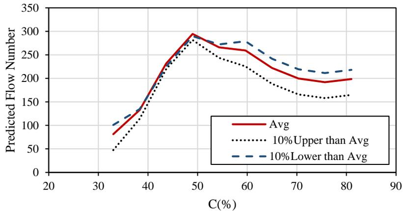
**Figure 4. The effect of coarse aggregates on the flow number of asphalt mixtures.**
