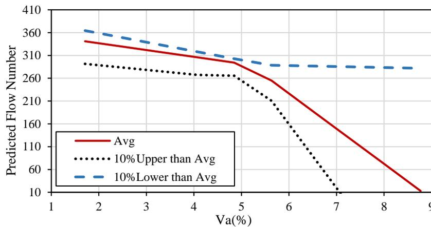
Figure 8. The effect of air voids on the flow number of asphalt mixtures.
