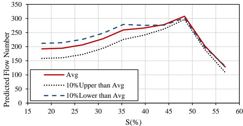
Figure 5. The effect of fine aggregates on the flow number of asphalt mixtures.
