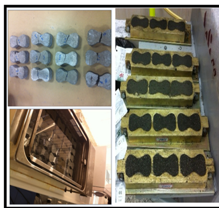
Figure 6. Samples and sample molds used for tensile strength test ASTM C307.
