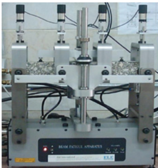
Figure 1. The schematic view of fatigue life test setup
