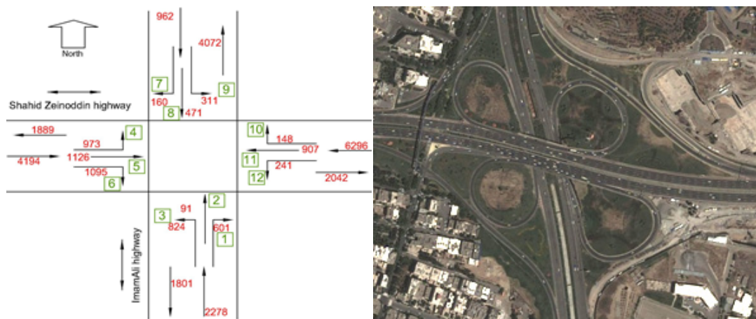
Figure 4. Shahid Zeinoddin – ImamAli interchange, Left: Traffic distribution statistics, Right: Aerial photo of the existing situation [Hexa CE, 2010]
