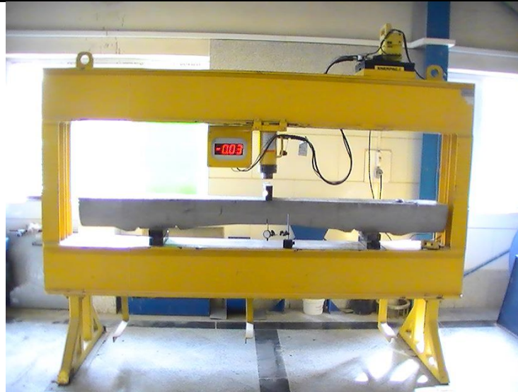
Figure 3. Three-pointed bending test with the load cell and the displacement gage.
