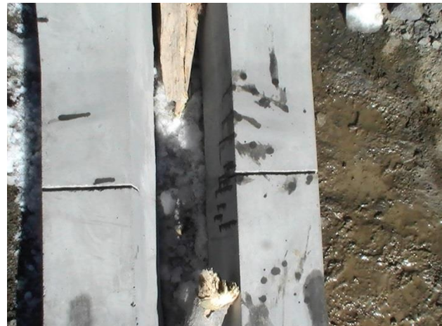
a. The center of the sleepers is painted before cutting. b. The center of the sleepers is cut. Figure 2. The center of the sleeper specimens.
