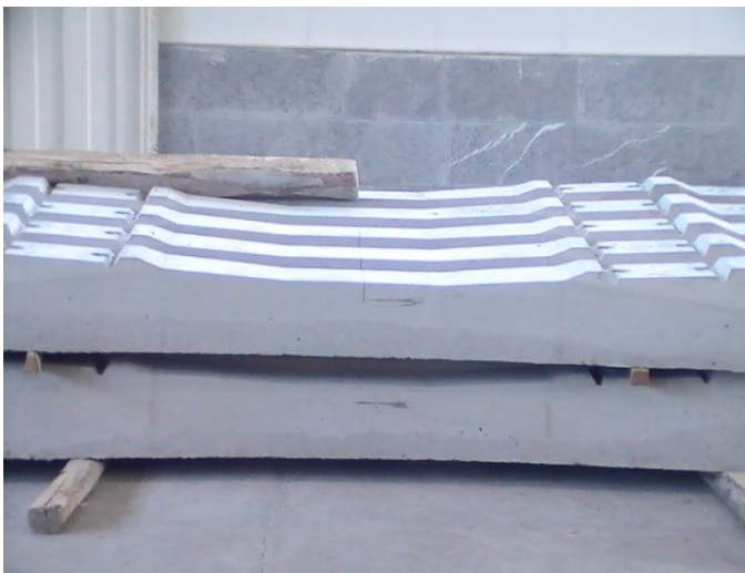
a. The center of sleepers is painted before cutting.
