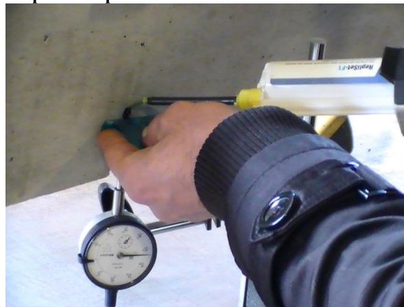
c. The Replica compound injection with Replica set.
