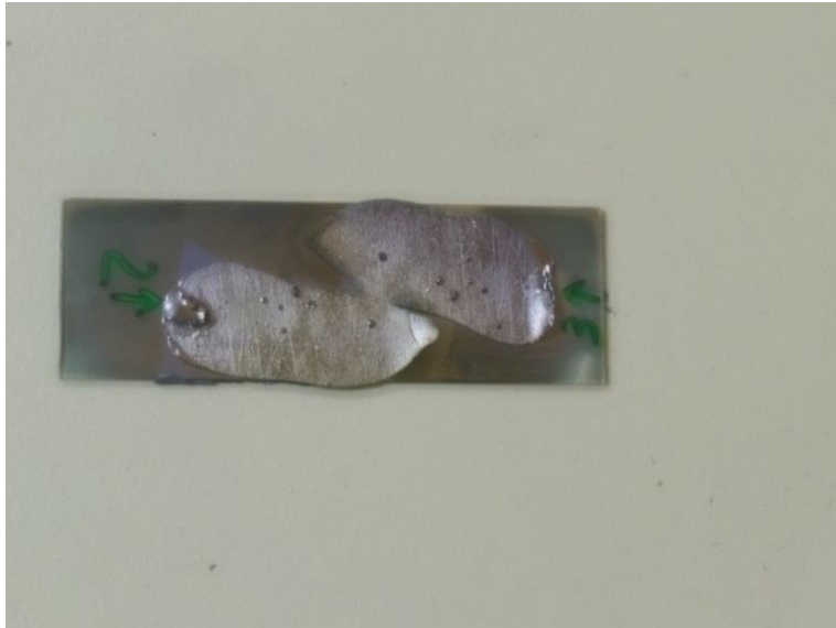
Figure 6. Covering the Replica sample with the thin layer of gold.
