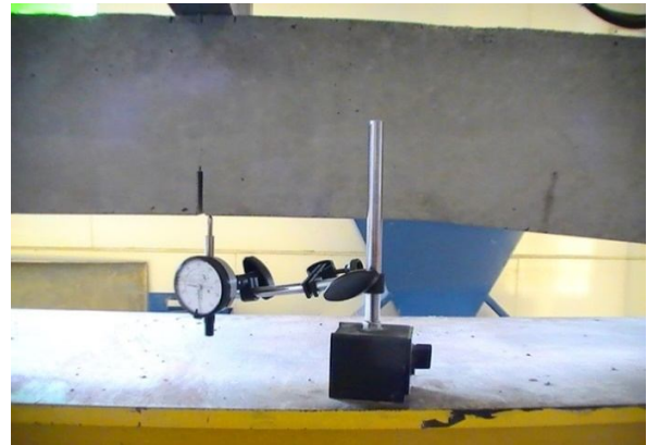
c. Displacement gage.
