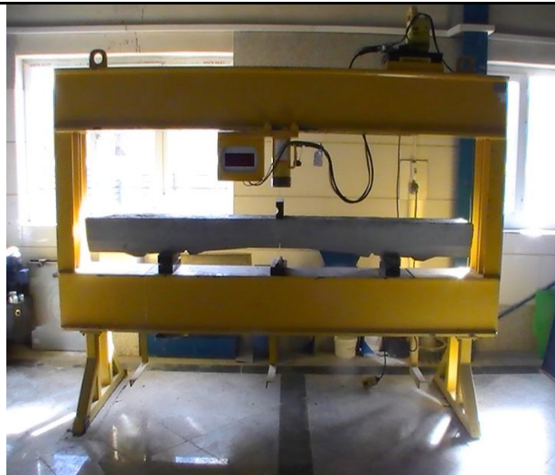
a. Three-pointed bending test with the load cell and the displacement gage.
