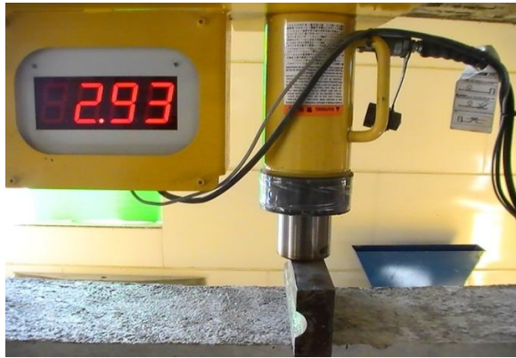
b. Digital load cell.
