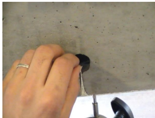
Figure 5. Separation of elastic hardening Replica from the cracks surface.
