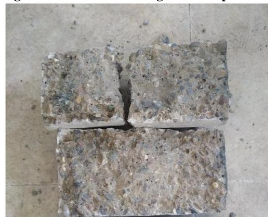
**Figure 4. Concrete Specimen after Tensile Strength Test**
