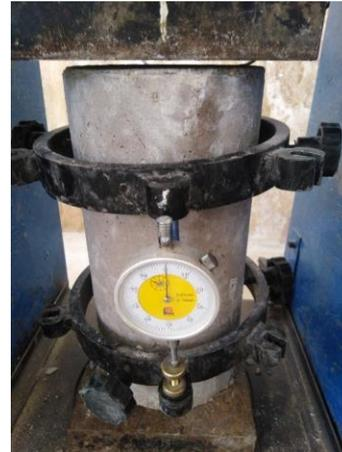
Figure 6. Concrete Specimen Undergoing Modulus of Elasticity test
