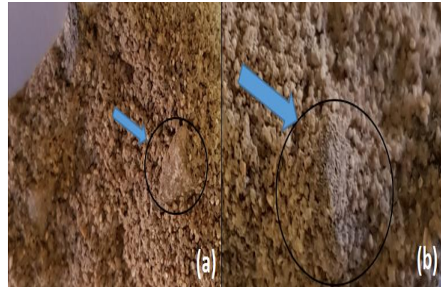
Figure 5. a) The FRAPA mixed with sand (lower magnification), b) The distribution of the aggregates among dune sand particles (in 15%)
