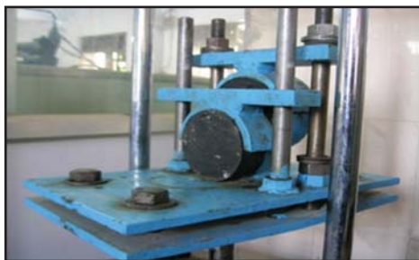
Figure 3. Close up photographic view of fabricated Inter-layer Bond Strength Testing Device
